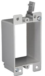
EZ10SOLV is a 1-gang, old work, low voltage EZ BOX used for low voltage installations in renovation (old work) residential and light commercial applications. The backless design is great for the large or deep low-voltage wiring needed for communications and cable installations.
